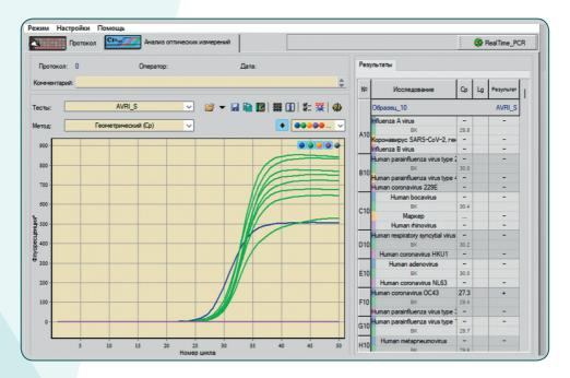
An example of the result of a PCR test using a detecting thermocycler of the «DT» series and related software: analysis of optical measurements
