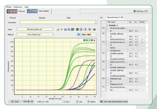
An example of the result of a PCR-assay using the «DT» series real-time PCR instrument and related software: analysis of optical measurements.
