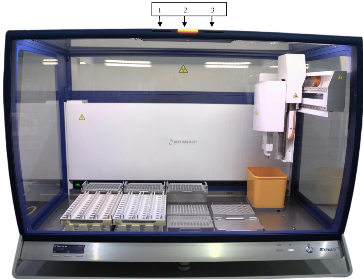
Figure 5 – Light indication of the current state of the instrument
