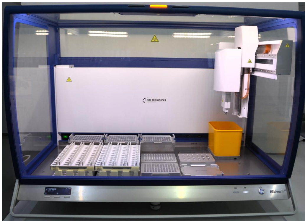
Figure 1 – Example of arrangement of additional equipment (accessories) on the DTstream 12M4 worktable
