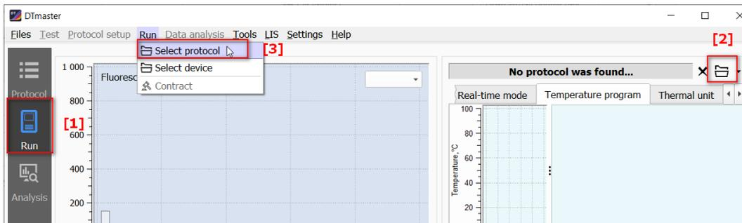
Figure 45 – Loading a previously generated protocol in the Run mode window
