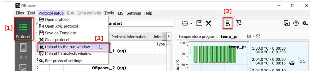
Figure 44 – Loading the protocol from the Protocol mode
