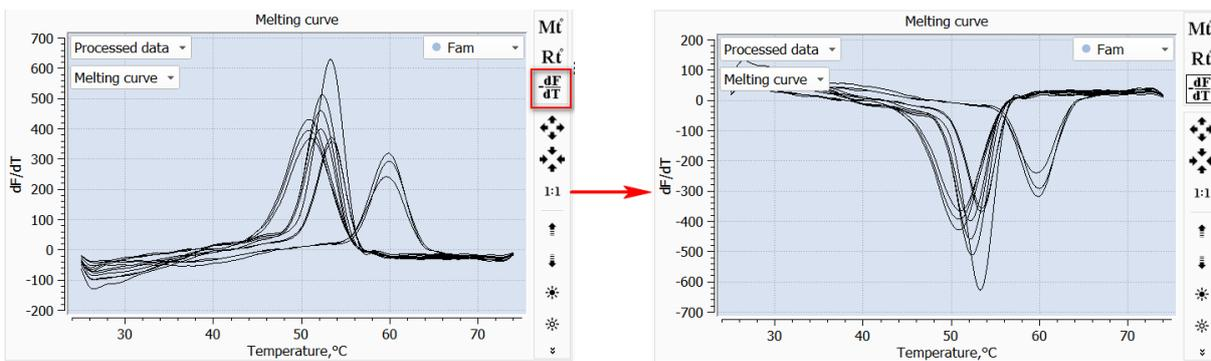
Figure 71 – An example of using the mode of melting curves inversion
