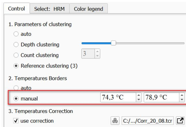
Figure 95 – Manual setting of the temperature limits
