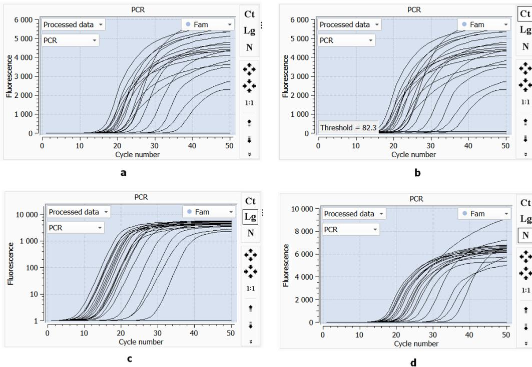
Figure 68 – Modes of viewing the graphs: a – with additional modes turned off; b – in the Ct mode; c – in the **Logarithm** mode; d – in the **Normalization** mode
