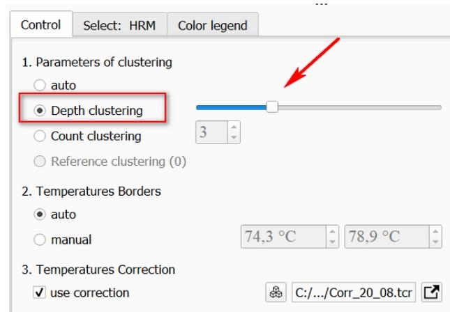
Figure 91 – Changing the **Depth clustering** parameter in the settings
