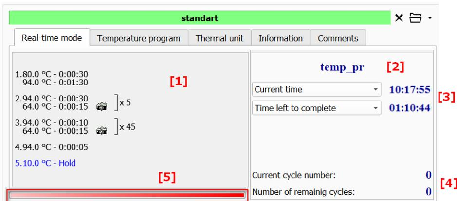
Figure 47 – The **Real-time mode** tab
