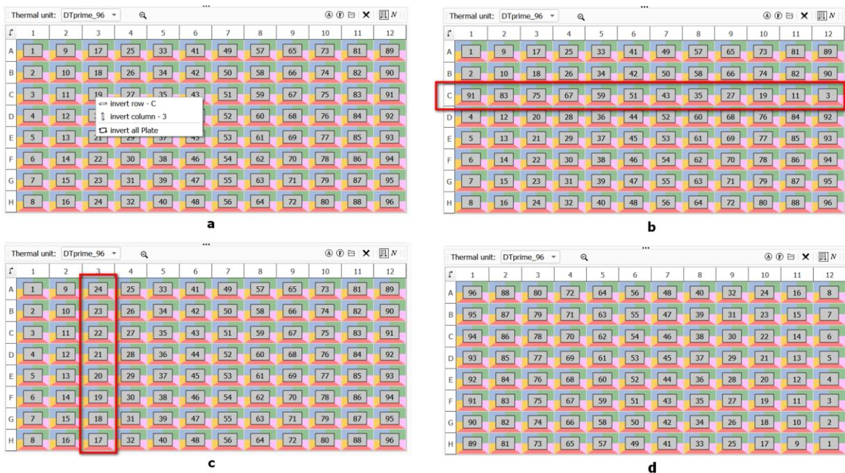
Figure 35 – Using inversion: a - options for inverting records available in the context menu; b - line inversion; c - column inversion; d - inverse of the entire placement table
