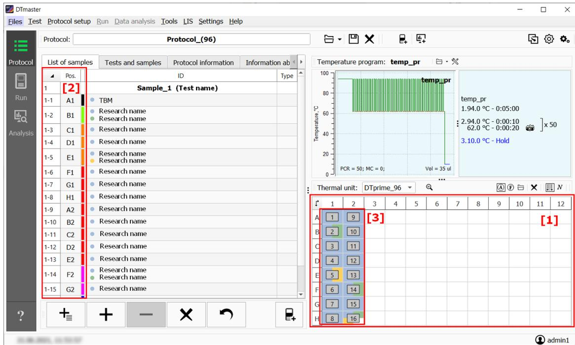
Figure 24 – Correspondence of the number of samples to the capacity of the thermal plate
