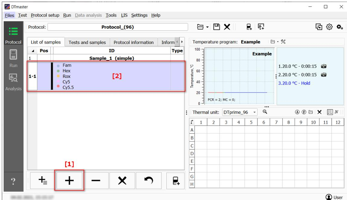
Figure 38 – An example of adding a test without using the **Test** option
