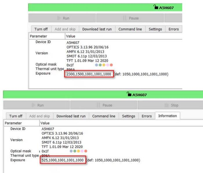
Figure 55 – Values of optical measurements exposure: a – before starting the analysis; b – after starting the analysis and applying the coefficients from the test settings
