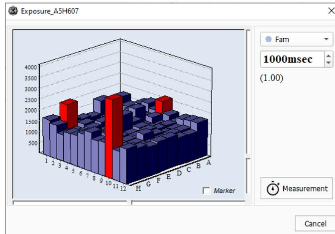
Figure 113 – Current values of optical measurements in three-dimensional coordinates for a given exposure
