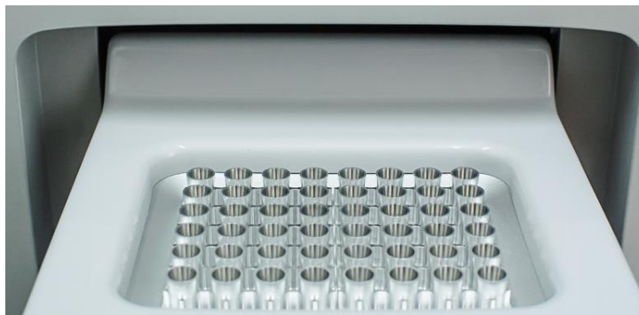
Figure 4 – Appearance of the thermoblock matrix in the extended position
