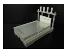
**Rods dispenser** is installed on the worktable of the devices in versions DTstream9 L1, DTstream9 L4, DTstream12 L1, DTstream12 L4, DTstream15 L1, DTstream15 L4 and is intended for placing cartridges with magnetic "rods" in it.
