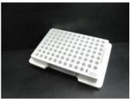
96-well for low profile strips, test tubes and microplates is installed on the worktable of device of all versions and is designed to be placed in the wells of the rack for strips, test tubes and microplates.
