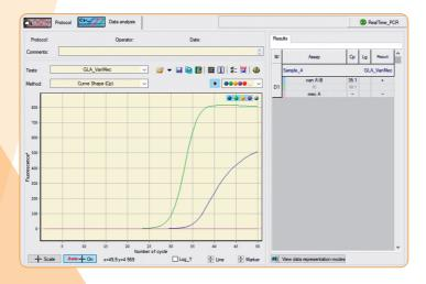
An example of the result of a PCR assay using a real-time PCR instrument of the «DT» series and related software: analysis of optical measurements.
